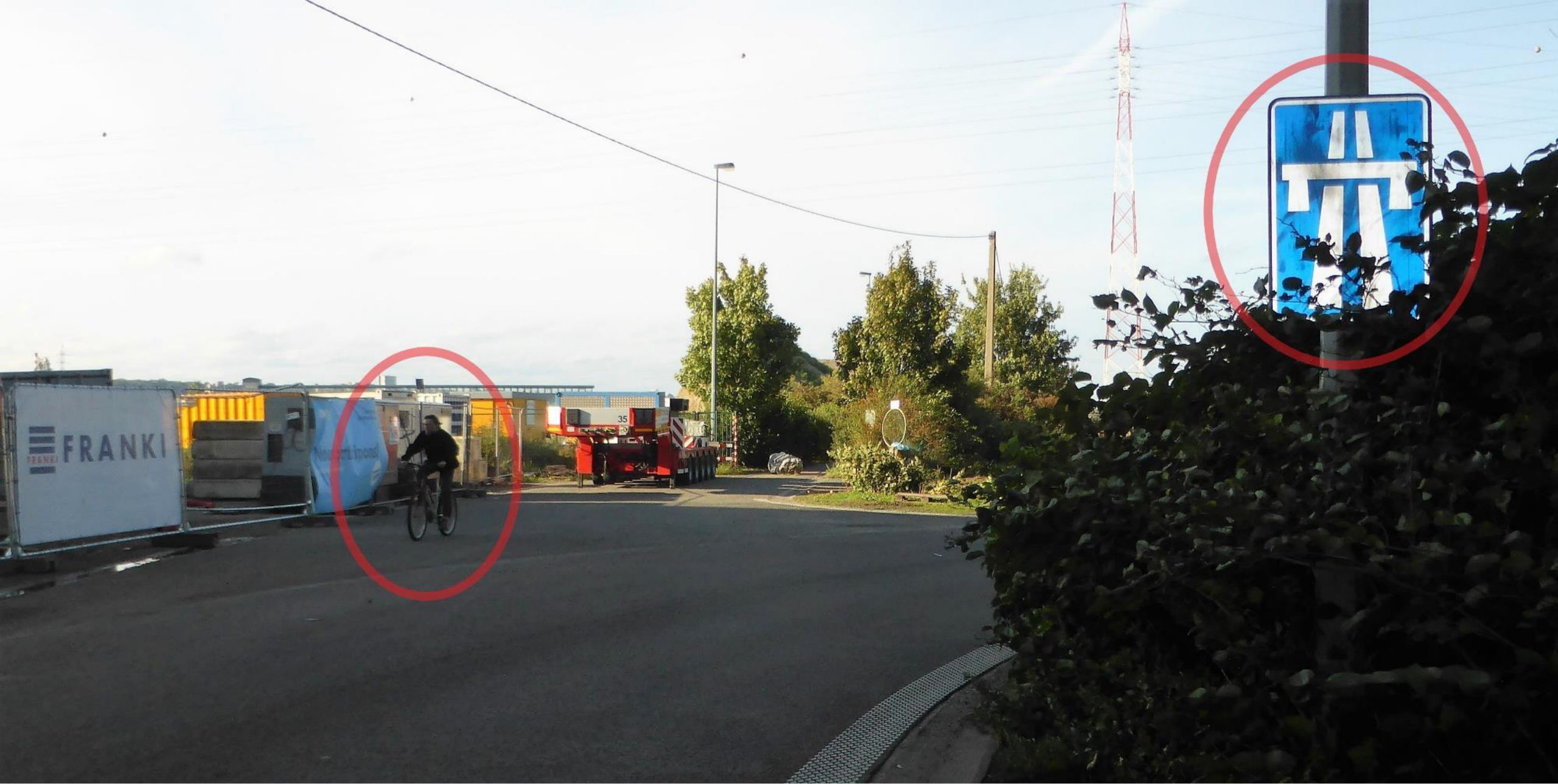
Dangerous: signing fault, cycle path connects to motorway ramp
